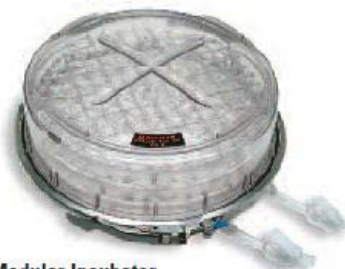
Fig. 05 | Sealed Modular Incubator Chamber
